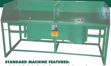
This dual-spindle assembly table allows two people to assemble up to 2,400 nuts per hour.
